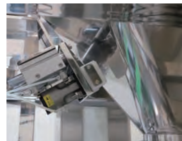
KIT introduces a vibrator in order to drop powder effectively.
