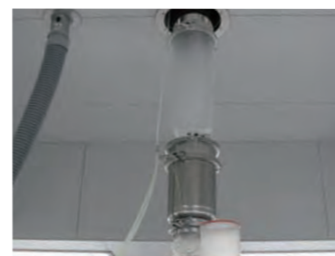
A balloon chute that gently drops product by putting air between the inner tube (made of polyethylene) and the outer tube.
