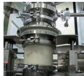
KIT introduces an automatic connecting expansion seal of silicone to prevent dispersion.
