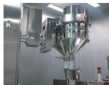
【Installed example】 A lifter which simultaneously ascends/descends and turns round two sanitary containers then injects.
