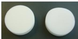
Figure 2. Compritol® 888 matrix tablet before and after 12h dissolution
