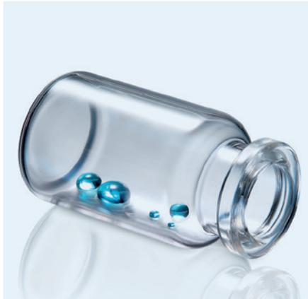
Silicization presence/absence and uniformity using colored water droplet test
