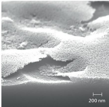
Delamination of the container wall by Scanning Electron Microscopy
