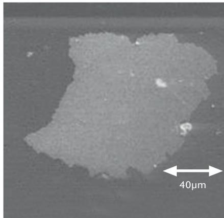
Flake-like particle (left) which is an Al-Phosphate rich material (right)
