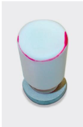
Dye penetration testing concerning glass container integrity
