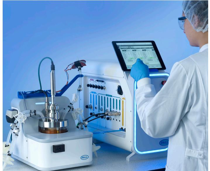
Process simplification, from vial thawing to final product, is at the heart of the iCELLis platform. As cells are immobilized in the fixed-bed (Figure 3), and the iCELLis system operates in perfusion / recirculation mode, no centrifugation is needed to harvest the cells. This benefit further simplifies the downstream process.
