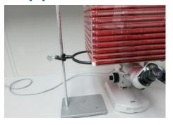
If the microscope stage is not capable of supporting the weight of the Cell Factory system, it is advisable to use an adjustable stand to support some of the weight of the Cell Factory system.
