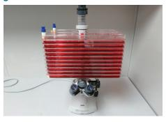
Place the Cell Factory system on the stage with the desired location to be visualized over the objective lens. If necessary, replace the light source or place an alternative light source above the Cell Factory system.
