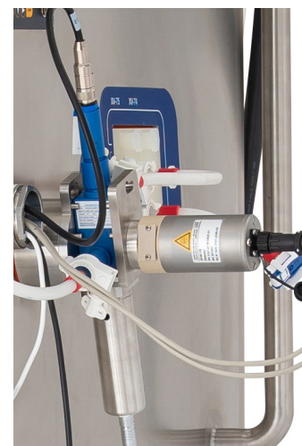
Figure 7. Post-column sensor pack with UV detector.
