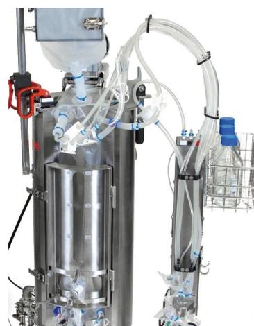
Figure 9. Cable/tubing management system.
