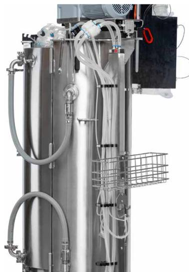
Figure 9. Cable/tubing management system
